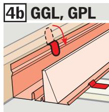
**ENGLISH:** Reposition sill flashing section and attach it to bottom frame with roofing nails provided.
