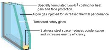
VELUX utilizes the latest technology in producing their own insulated glass to ensure that it meets the highest efficiency standards. Comfort Glazing ensures that VELUX products provide unparalleled protection against heat gain and heat loss, fading and condensation. Comfort Glazings are also superior to plastic because it is more energy efficient, more durable, and reduces external noises (rain). Also, unlike plastic it will not discolor, leak or allow drafts.
