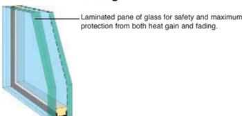
**Comfort Glass** allows a broad spectrum of light into the home and is extremely durable and essentially maintenance free. Plastic diffuses light and obscures views, and may degrade with time and exposure to the elements. Comfort Glass consists of tempered safety glass double-coated with Low-E, dual-sealed and injected with Argon for energy efficiency.
