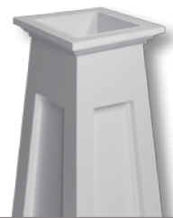
Recess is 5/8" deep and corners are 1/4" rounded.
