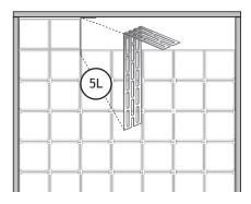
M. Screw the short leg of the anchor to the top of the opening.
