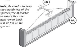
B. Place a "FLAT" spacer on top of the first and last block of the previous row where they meet the side channels.
