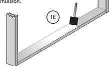
If using Weldbond<sup>®</sup>, apply mortar to the surface before it cures. Otherwise, let the treated area set up and cure before installing the first row of block.
