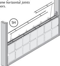
**Note:** If using 12" x 12" nominal size glass block, panel anchors and panel reinforcement should be installed on top of every row, except the top row.
