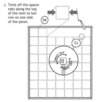
K. Install two blocks, buttering both vertical sides of the second block before installing.
