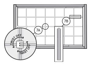
A. Twist off the spacer tabs on both sides of the panel.
