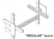
• Where block meet the side perimeter channel, clip off both sets of smooth legs. Twist-off tabs remain in place. File off any burrs so the spacer will lay flat. These are called "FLAT".
