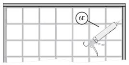
F. If your glass block panel will function as a shower wall, after about a week, coat the mortar joints on both sides of the panel with tile grout sealer for mold and mildew protection. Repeat this every two to three years.
