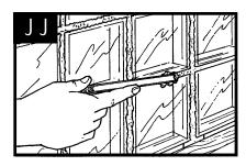
• Take the striking tool and run it with moderate pressure over all the joints. It is best to strike all the horizontal joints first, then the vertical joints, so that the pattern is uniform (Illus. JJ). Striking removes
