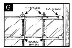
Use the "H" and "FLAT" spacers as shown (Illus. G), when installing the next to the last row of glass block.
