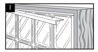
Around the perimeter use the glass block sealant to seal between the glass block and channel and to seal the top channel to the frame at the head. For exterior panels or wet areas, you should also seal between the channels and the framing. You may want to cover the edges of the channel with trim molding depending on the look you're trying to achieve.
