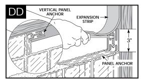
Trim expansion strip for length based on the distance between anchors with scissors or utility knife. The expansion strip width should be trimmed to 2<sup>1</sup>/<sub>8</sub>" for Thinline<sup>™</sup> Series block and 2<sup>7</sup>/<sub>8</sub>" for Premiere Series block. The length should also cover the anchor short arm. Strips are installed between the anchors for the full length of the jamb and head (Illus. DD).
