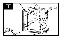
**NOTE:** Preparing mortar is an important step. If you have ever laid brick or concrete block, be aware that **glass block are nonabsorbent** and, accordingly, the mortar must be much less moist. The consistency should be spreadable, but not dry to the point of separating or crumbling. When mixed to its proper consistency, mortar should stick to the edges of the block when it's turned on edge. Mix what you think you'll use in about an hour.
