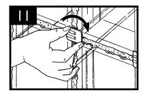
Remove excess mortar from the block faces using a damp sponge. Be sure to rinse the sponge frequently. Try not to let any mortar on the block faces dry or set before attempting to remove it. Don't be concerned about the dry film that remains on the block, it will be cleaned off later. Be sure you don't use abrasive materials for this cleanup, since they scratch the glass surfaces.
