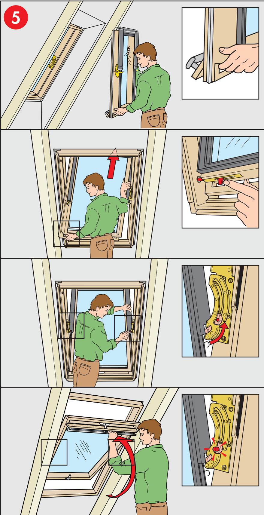
**English:** Replace sash, if removed earlier. The push button is automatically released when the sash is rotated to the closed position.
