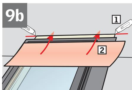
**ENGLISH:** To allow for proper drainage, interweave roofing underlayment as shown in 9a for new construction applications. For retrofit applications, interweave roofing underlayment as shown in 9b.
