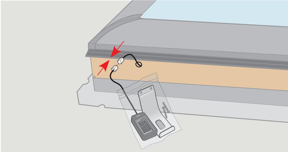
**ENGLISH:** Connect the rain sensor as shown and leave the bag with its contents on exterior side for attachment during installation of flashing. Make sure that the wire and the bag is protected while installing the skylight, wrapping the frame and installing the flashing.
