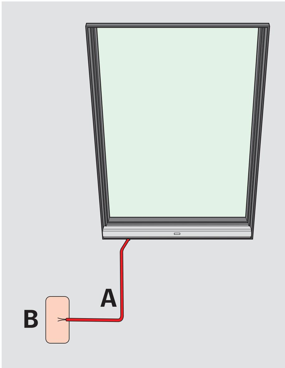
**ENGLISH:** A junction box or an outlet box (not provided with skylight) is required for connection of the 20 ft/6 m skylight wire.
