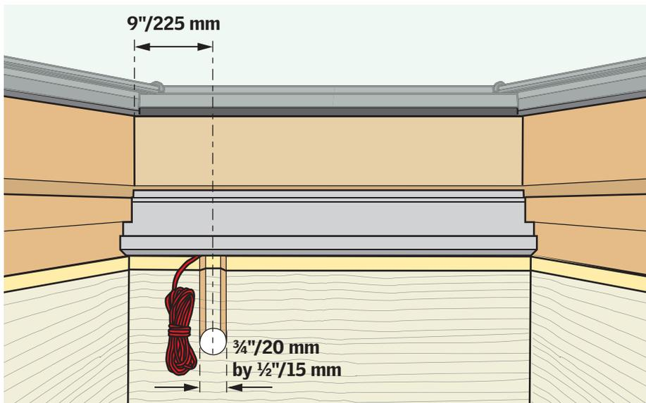
**ENGLISH:** Prepare the framing for electrical wire (applies to VSE only). Refer to national Electric Code for wire routing details.
