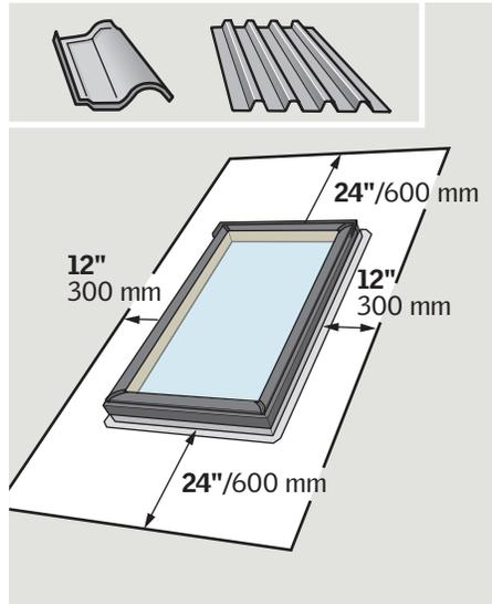
**ENGLISH:** Maintain illustrated clearances between skylight frame and critical areas such as valleys, ridges, slope changes and roof-to-wall-intersections.
