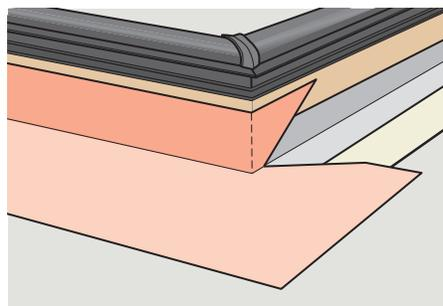
**ENGLISH:** To ensure waterproofing, skylight frames should be completely wrapped in VELUX adhesive skylight underlayment supplied with the flashing. This underlayment must be applied before installing the flashing.
